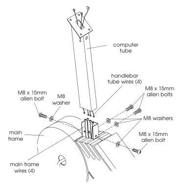
Figure 6 - Install Computer Tube
